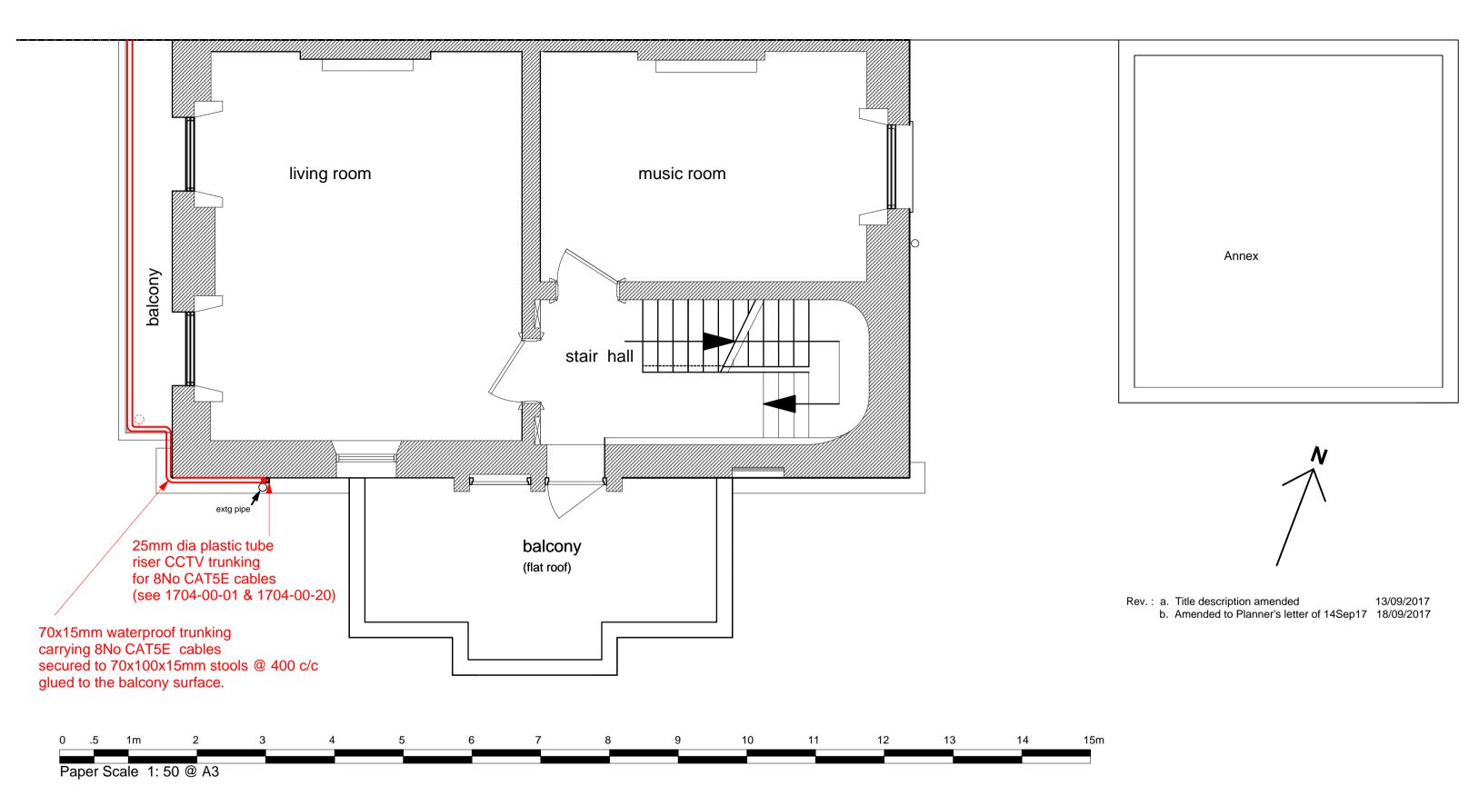
"Installation of 4x pairs of CCTV security cameras mounted on the underside of the balconies at Nos. 1, 6, 11 and 17 Regents Park Terrace, connected by a black cable duct running along the top of the balcony terrace from Nos. 1 to 17"
