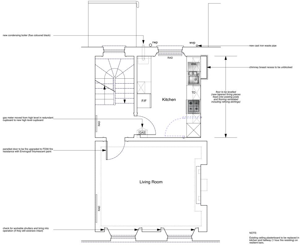
Existing, flush internal doors to be replaced with solid timber flush fire doors.
