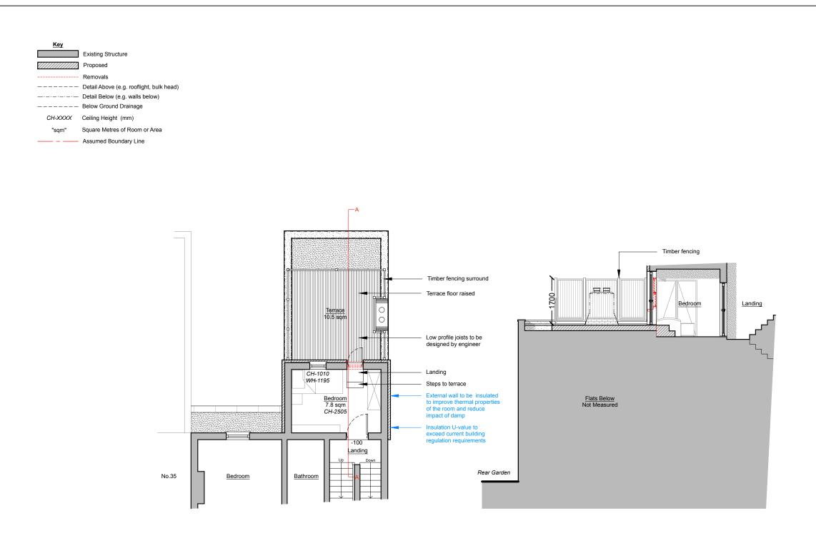
Rear Second Floor Plan As Proposed - Scale 1:100
