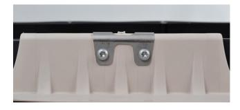
A metal clamp, perfectly matching with the shape of the Sika SolarClick, is used in case of higher temperatures or larger horizontal loads. It is going to be fixed through the mount's web by 2 screws which are delivered with the clamp.
