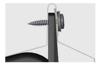
Cross-section of the wind deflector screw position.
