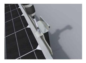
Fasten the 4 module clamp screws with a torque of 2 Nm.
