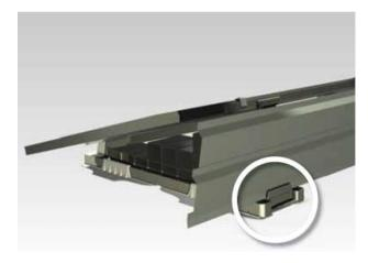
Insert the wind deflector sheet in the lip at the rear bottom of the rack. The sheet must fit flush with the outer edges of the module row.
