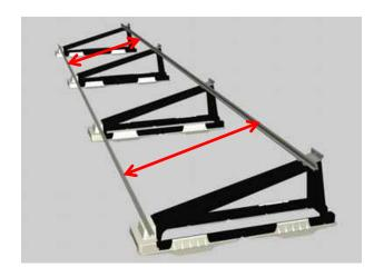
Insert assembling jigs with the width of a module (see red arrows let) on both sides between the mounting rails in order to establish the exact distance to one another, and then remove the jigs.
