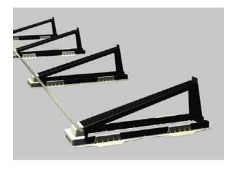
Once all mounting racks are firmly connected to the assembly rail, these are placed back on foot by turning them by 180°.
