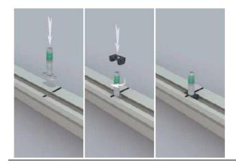
Place the hammer-head screws (M10 thread) on the marked places into the groove and twist them a little clockwise to prevent them from falling out. Place the twist protection on the hammer-head screw. Now fix the twist protection in the groove.
