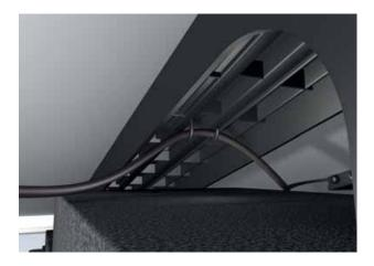
Insert the bundled cables into the mounts in the mounting racks. The cables shall not be allowed to swing, and the connectors may not be left on the roof as it may lead to leakage current due to ponding water.
