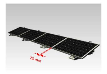
Insert the remaining modules with a distance of 20 mm to the adjacent modules. The junction boxes of the modules should face to the same side.
