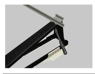
Tighten the nuts with a torque of 15 Nm.
