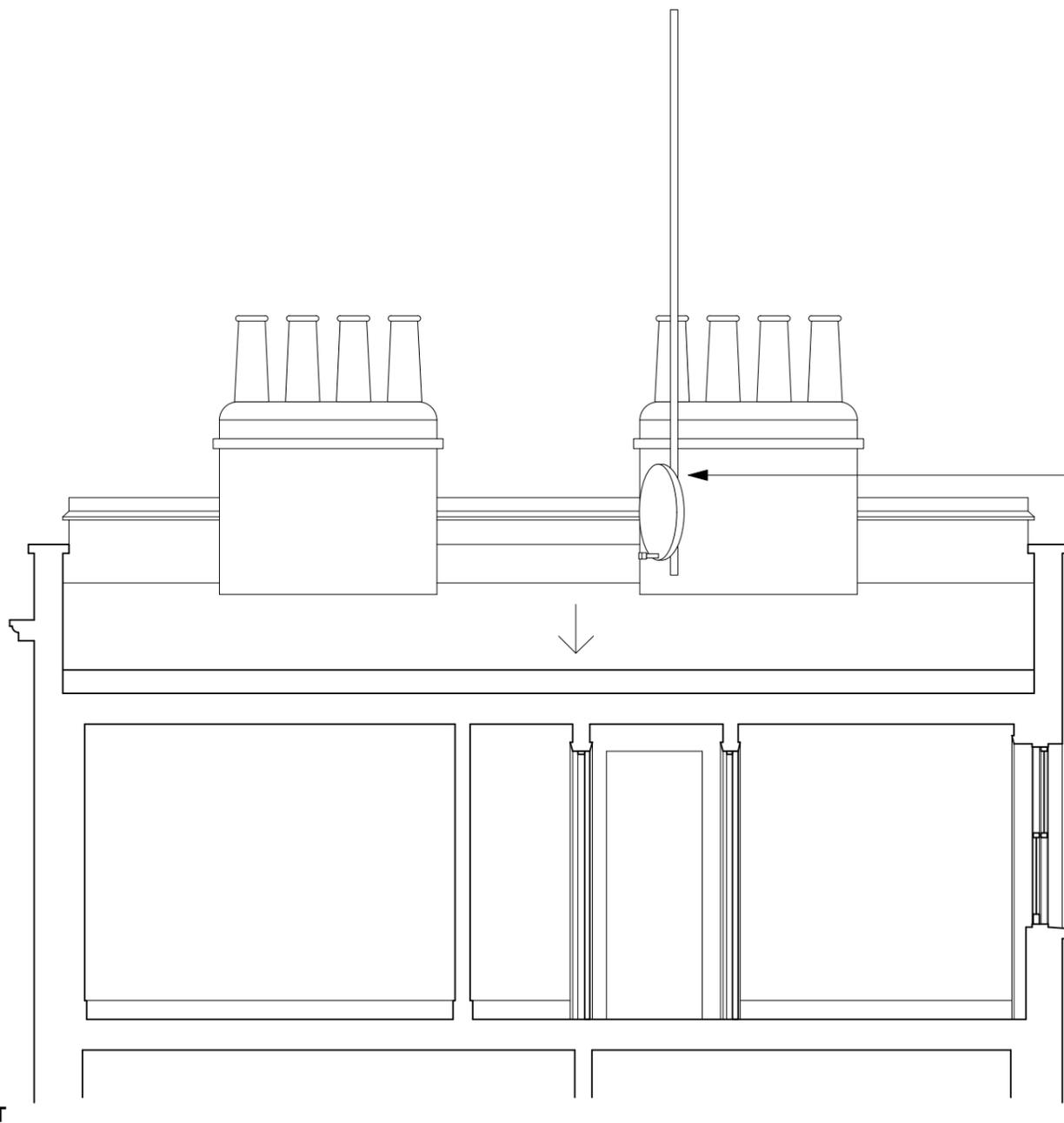
Integrated Reception System (IRS) comprising 78cm diameter shared satellite dish and FM, UHF & DAB aerials. To be painted black and to be located on rear section of chimney stack as far below ridge as practicable, so as to minimise its effect on the property and on the amenity of the area.
