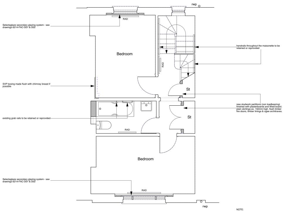
Existing ceiling plasterboard to be replaced throughout second floor (1 hour fire resisting) on resilient bars.
