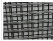
UNIT BACK PANELS STEEL WELDED MESH - FINISH TO MATCH BLACKENED STEEL FRAME WORK SAMPLE SUPPLIED BY CONTRACTOR. AGREED UPON BY DESIGNERS AND CLIENT.
