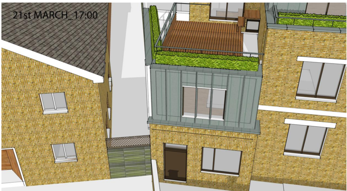
Extent of overshadowing at 1700hrs
