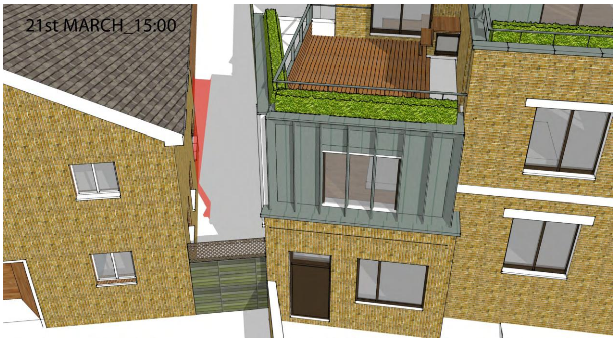
Extent of overshadowing at 1500hrs
