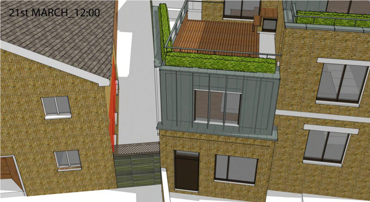
Extent of overshadowing at 1200hrs
