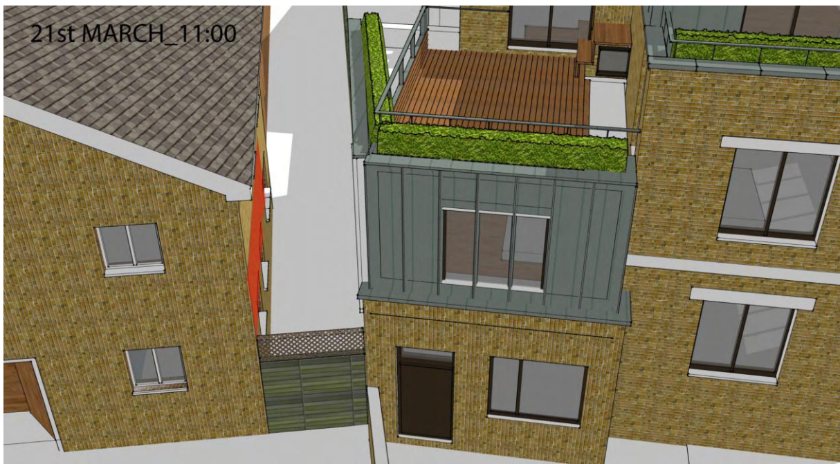
Extent of overshadowing at 1100hrs
