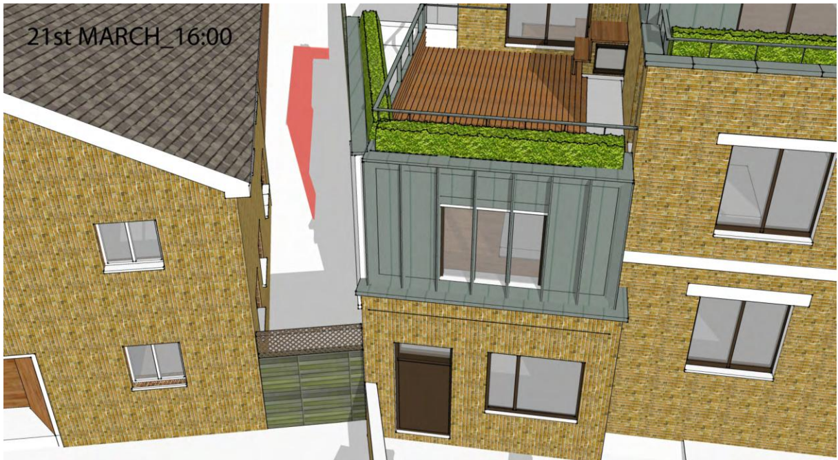
Extent of overshadowing at 1600hrs
