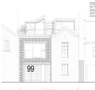
PREVIOUS BRICK ELEVATION TREATMENT
