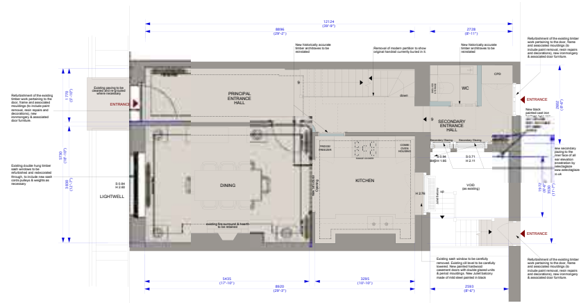
Proposed Ground Floor Plan - PR.101
