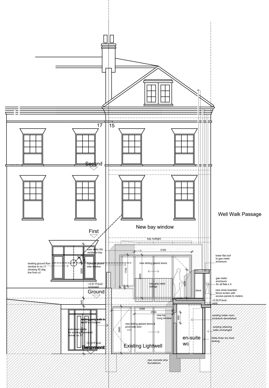
Proposed Rear Elevation showing no.17 basement annex
