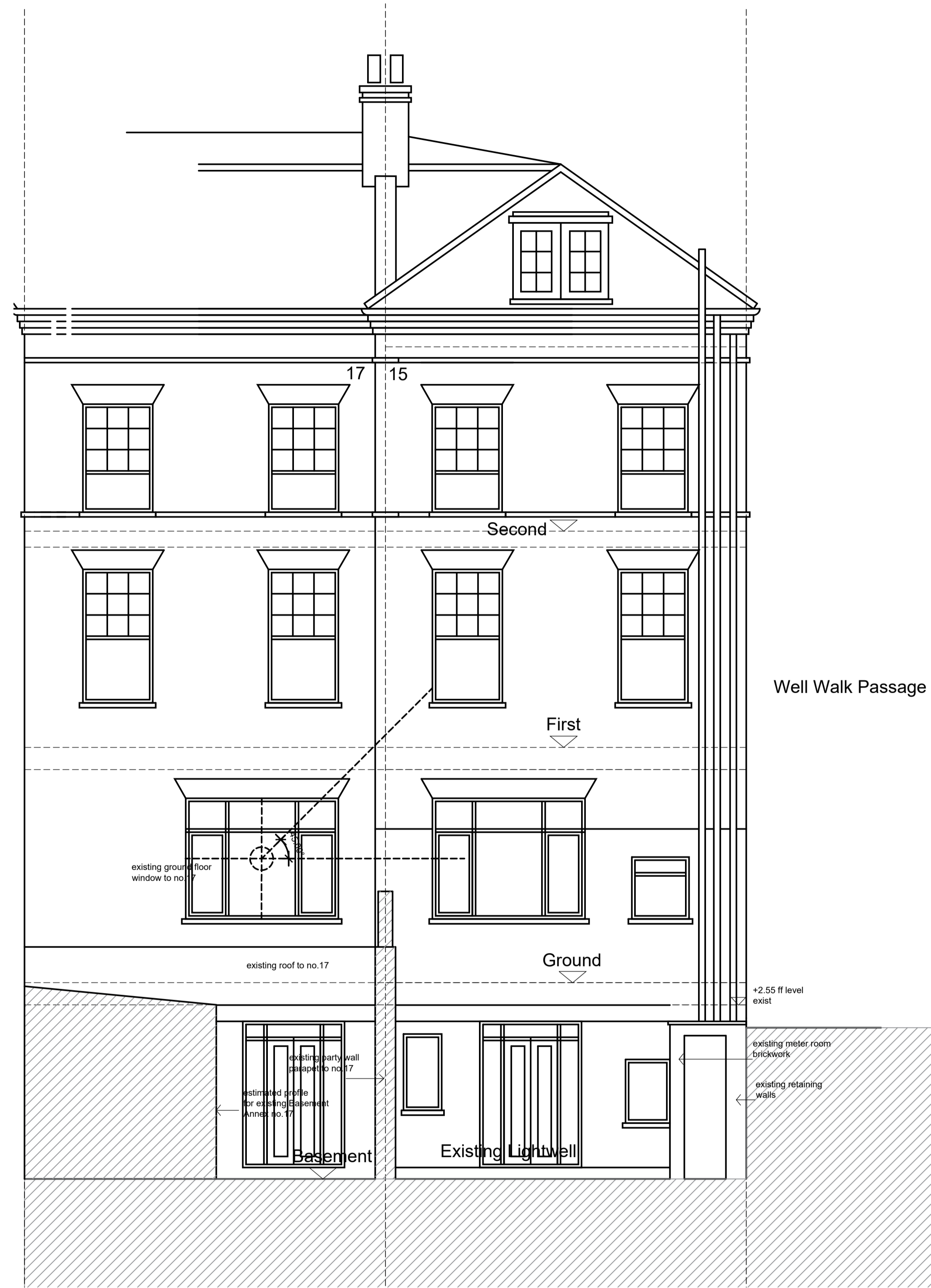
Existing Rear Elevation showing no.17 basement annex
