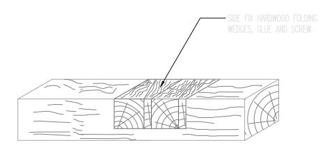
NOTCH REPAIR DETAIL FOR LONG NOTCH
