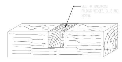
NOTCH REPAIR DETAIL 2
