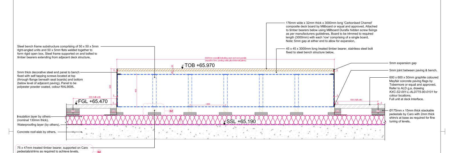
DETAIL 01: LONG SECTION THROUGH DECK BENCH INTERFACE WITH PCC PAVING
