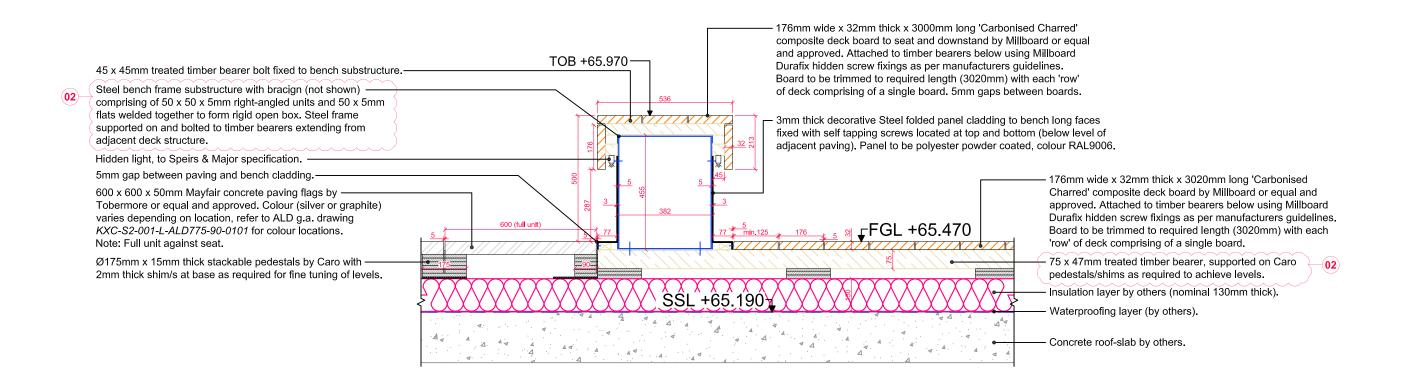
DETAIL 01: SECTION THROUGH DECK BENCH NTERFACE WITH PCC PAVING AND DECK
