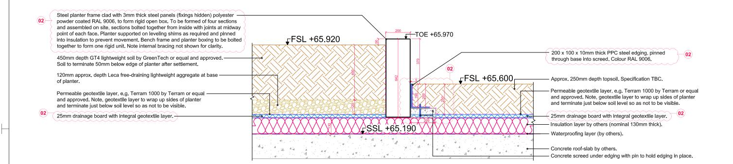
DETAIL 01: SECTION THROUGH HIGH PLANTER INTERFACE WITH LOW PLANTER
