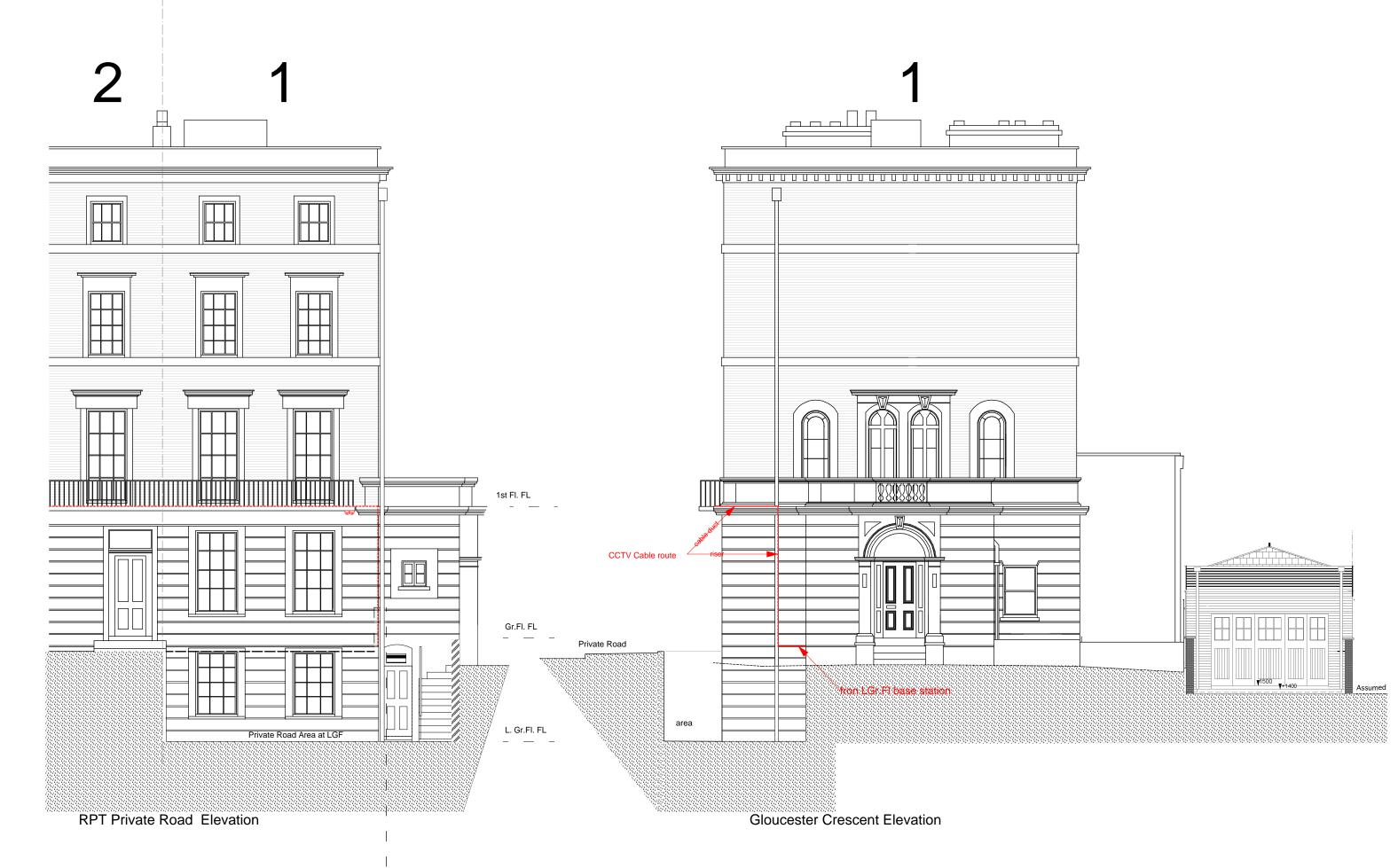
1 Regent's Park Terrace NW1 7EE- ELEVATIONS Proposed CCTV cameras installation cable route **REGENT'S PARK TERRACE NW1**
