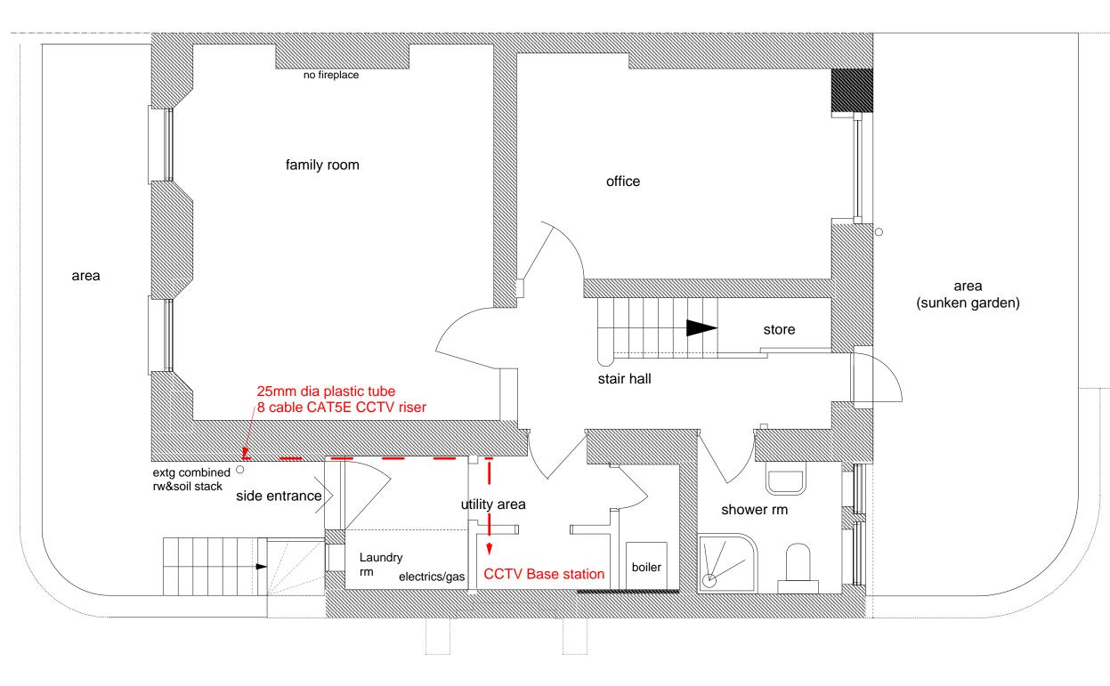
Basement Plan (1 Regent's Park Terrace NW1 7EE) Proposed CCTV cameras installation Base Station/cable route **REGENT'S PARK TERRACE NW1**
