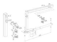
LOCINOX - www.locinox.com SAMSON ADJUSTABLE GATE CLOSER Adjustable closing speed & closing pressure Closing speed unaffected by humidity and temperature changes Adjustable freerun for perfect closing (final snap) Robust design Especially designed for exterior use: rain & frost-proof Designed with rustproof materials Fixing: Anti-theft & vandalism proof Fast and easy fixing: Quick-Fix Min. opening angle 90° (depending on the mounting situation) For left & right turning gates Tested to -30° C
