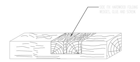
NOTCH REPAIR DETAIL FOR LONG NOTCH FOR NOTCHES GREATER THAN 25mm DEEP.
