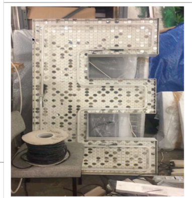
S1 SIGN REFERENCE IMAGE SIGN TO BE CONSTRUCTED WITH A FOLDED POWDER COATED STEEL TRAY W/ SEQUIN DISKS MOUNTED TO FRONT FACE. AS NEON LIGHTING IS NOT ALLOWED, ALLOW FOR A CONCEALED LED STRIP LIGHT TO WRAP AROUND "E" SIGN PERIMETER AND WASHER LIGHT OVER SEQUINS. NOTE: ALL "E" SIGNS ON THIS DWG TO BE HOUSED WITH IN THE INTERIOR OF THE BUILDING / BEHIND THE GLAZING.
