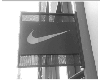
S8 SIGN REFERENCE IMAGE SIGN EXAMPLES SHOWN TO BE CONSTRUCTED WITH METAL MESH & SOLID STEEL SHEET PORTION. ALLOW TO POWDER COAT ALL TO PREVENT RUSTING & CONCEAL ANY MANUFACTURER IMPERFECTIONS, AS PER REF IMAGE ABOVE BY NIKE.
