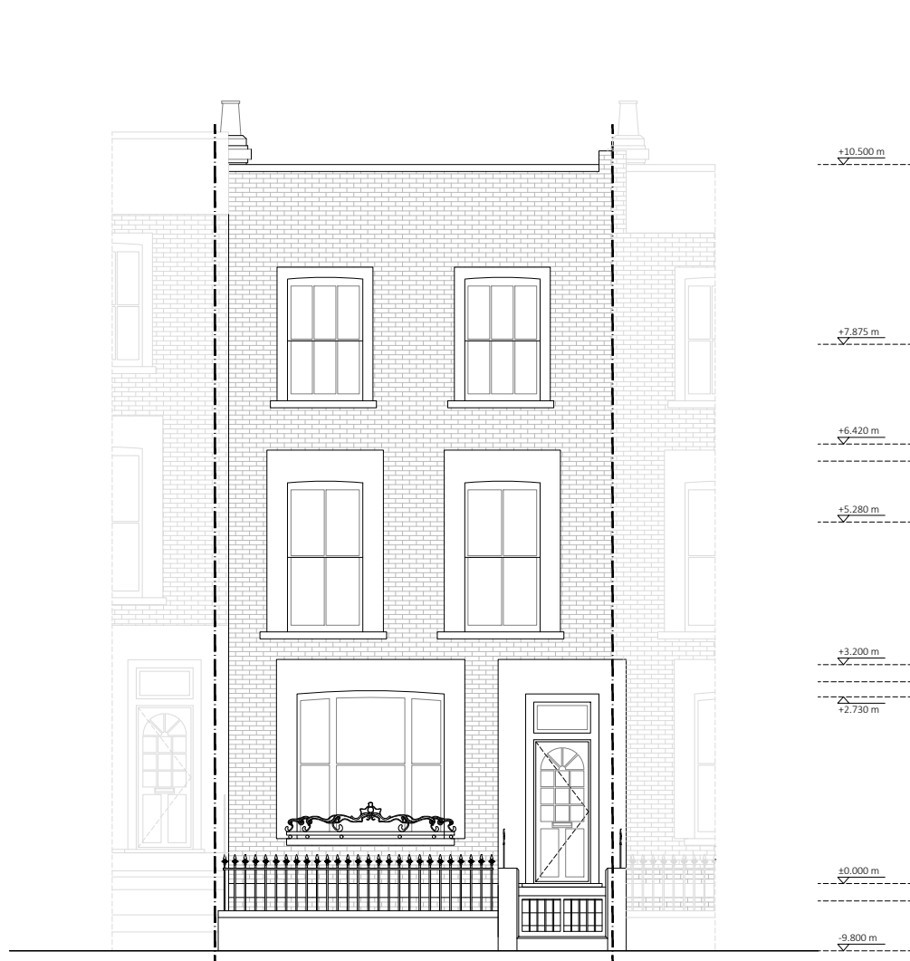
EXISTING FRONT ELEVATION
