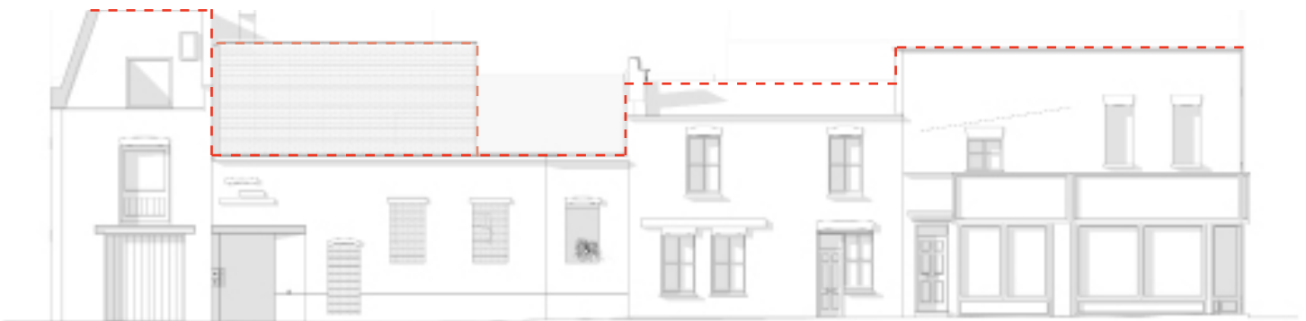
Front Elevation - Variety and difference in roof-line, 'shoulder' of the existing wall retained, roof extension set back
