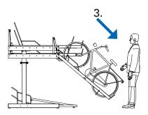
3. Lift the rear bicycle wheel out of the rear support and roll the bicycle off the cycle rack
