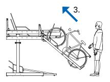
Place the front wheel of your bike onto the rack and wheel your bike along allowing the rear wheel to sit in the recess at the front
