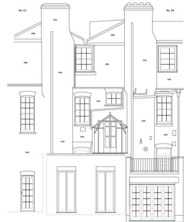
SOUTH-WEST ELEVATION (Rear) A13.03m
