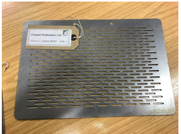
MATERIAL TO GATES IS PERFORATED METAL, PPC COATED 7022 TO MATCH METALWORK GENERALLY
