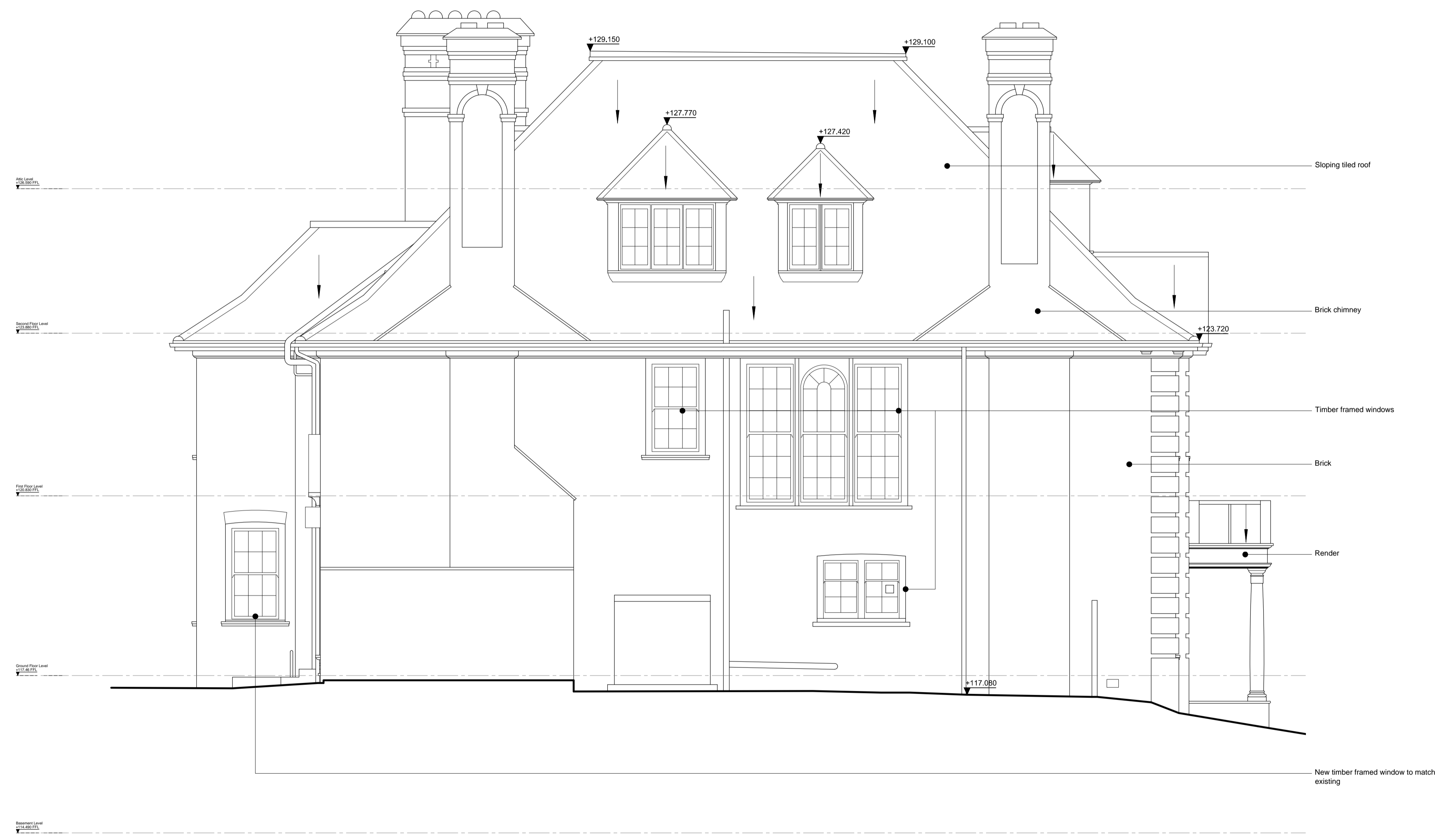
01 Proposed Side Elevation - D D(0)2703 SCALE: 1:50
