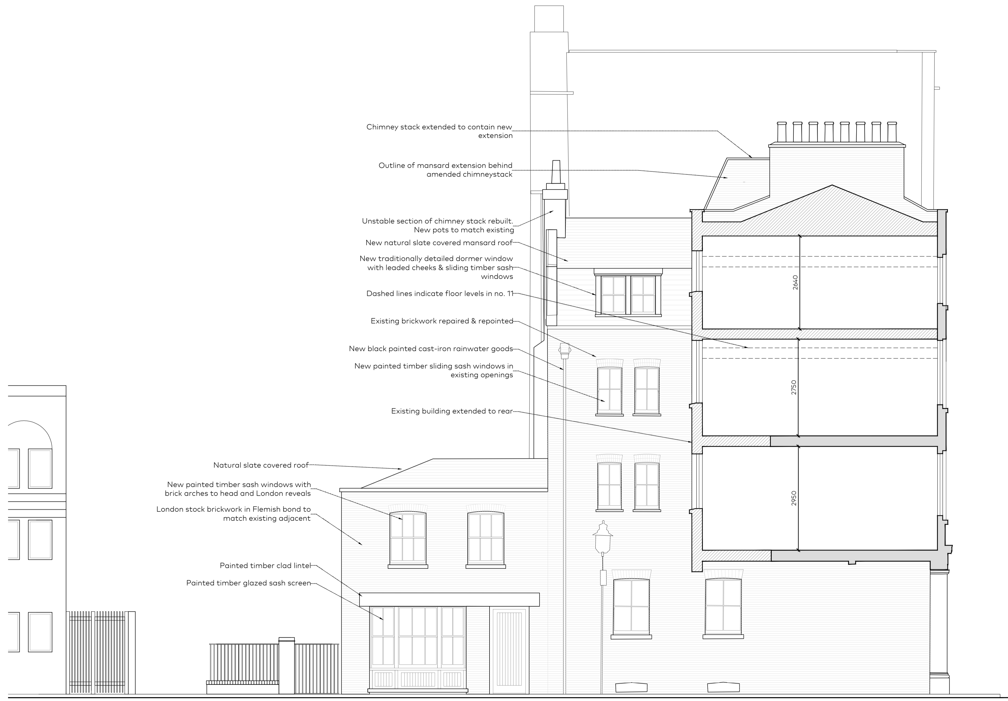
02 Partial Section CC As Proposed
