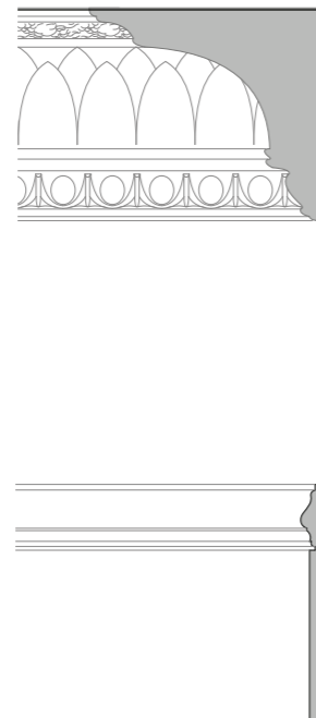
Fig 21: Existing Historical Cornice- Original fibrous plaster cornice with 4 elements; twin ogee and anthemion motif to ceiling, scotia and torus roll, finely decorated cavettoof interlocking flower and leaf pattern with torus roll and egg and dart to wall -Room 4101 & 4109 -
