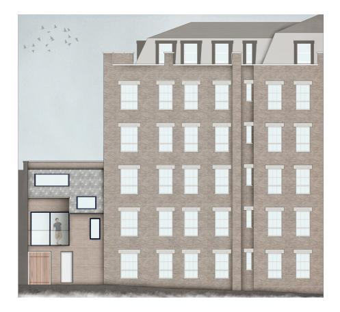
To the rear the elevation has been set inboard of Wells Court rear elevation ensuring the surrounding buildings are not overshadowed. At first floor level part of the rear elevation has been stepped inwards to form a small balcony space and with the rear section of roof being pitched the building profile maximises on allowing light into the rear courtyard.
