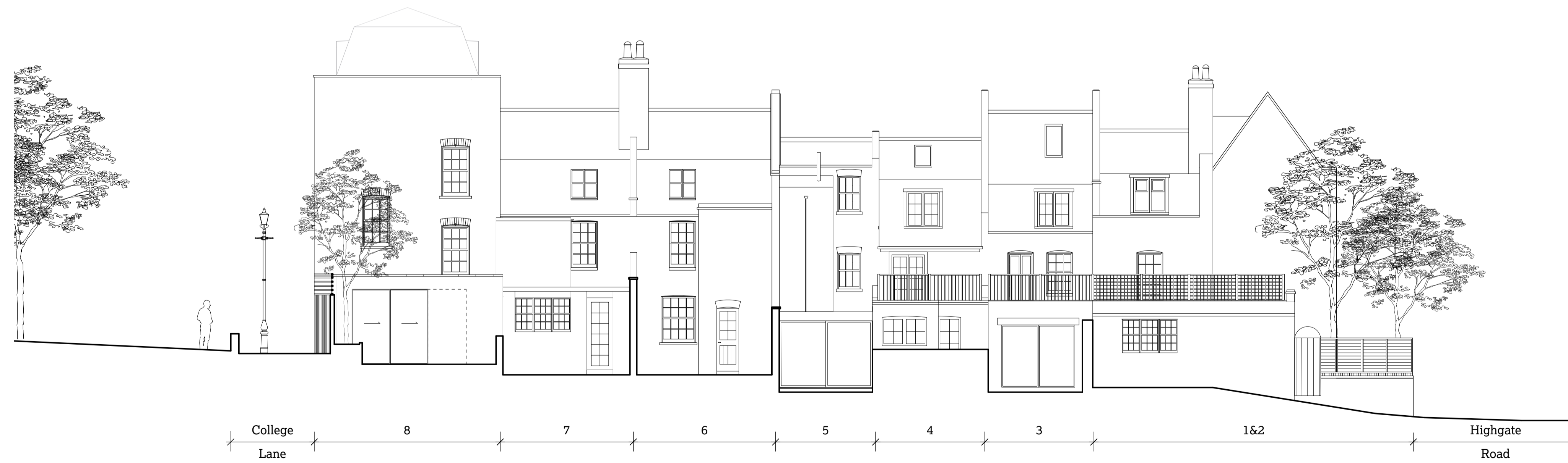
1 Proposed Little Green Street elevation (north side) 1:100
