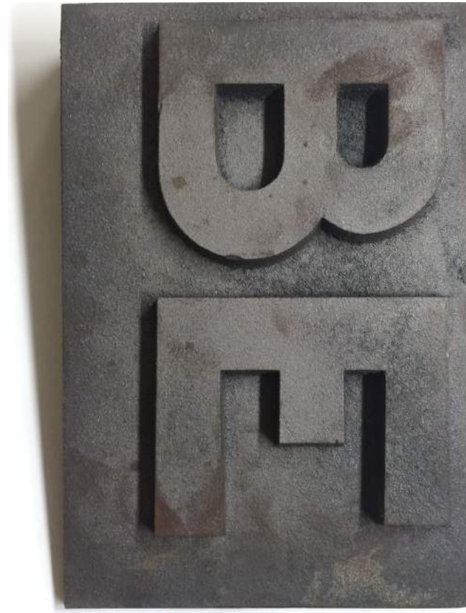
Figure 6.2c Sample main inscription cambered extrusion
