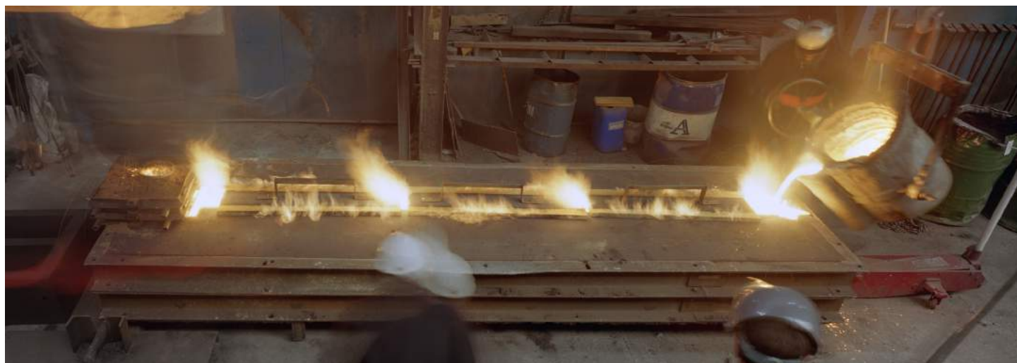
Figure 6.1a-c Casting process for the stainless steel stellae of the National Memorial
