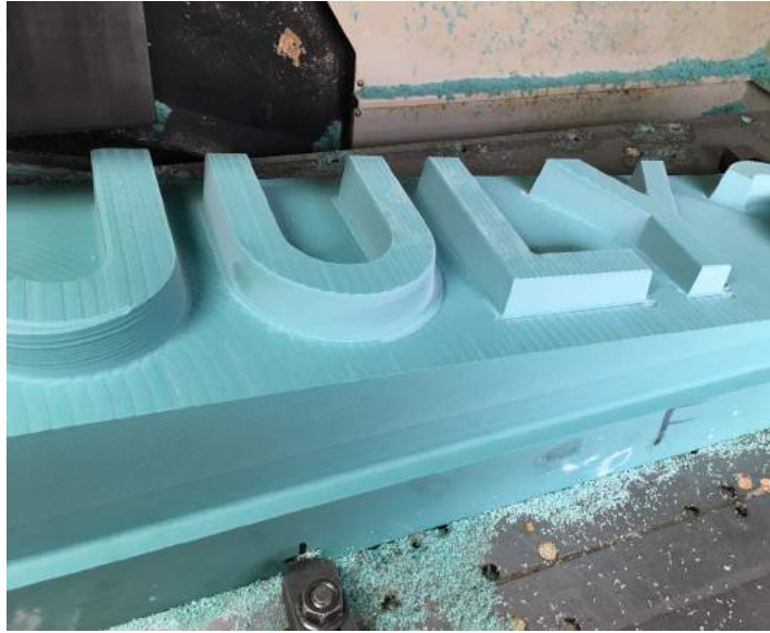
Figure 6.3a CNC fabrication of pattern for 7 July 2005 sample cast.
