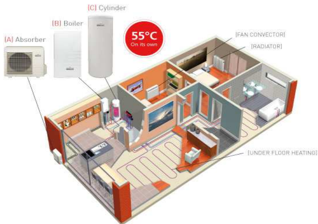
Figure 8: Standard domestic ASHP system layout
