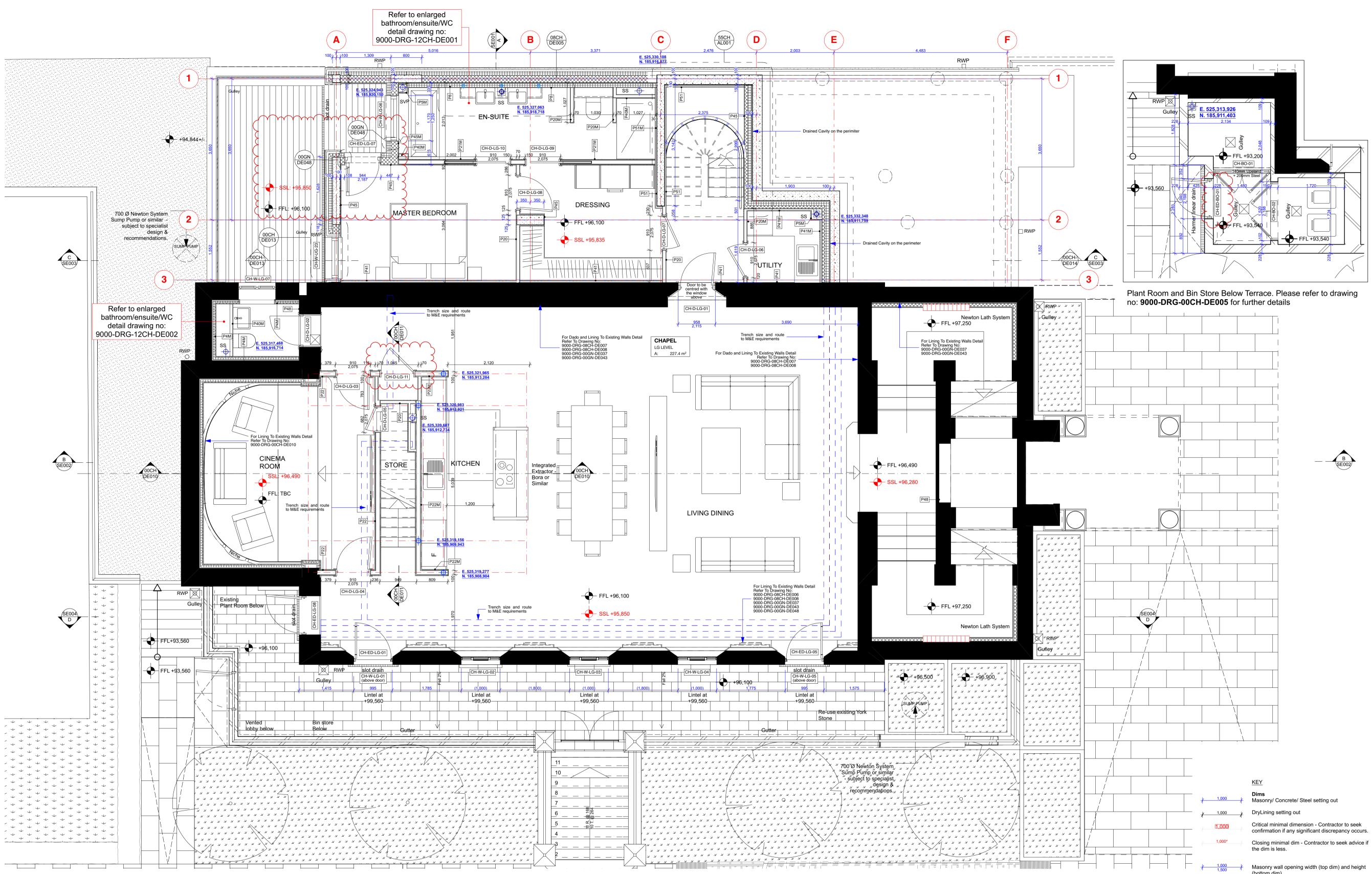
Finishes Legend : External and Separating Wall Lining Types: Type P1. External Metsec Wall - 2 layers of 15mm British Gypsum Soundbloc on Vapour Control layer. All joints to be taped and jointed, giving a smooth and seamless finish ready for decoration.
