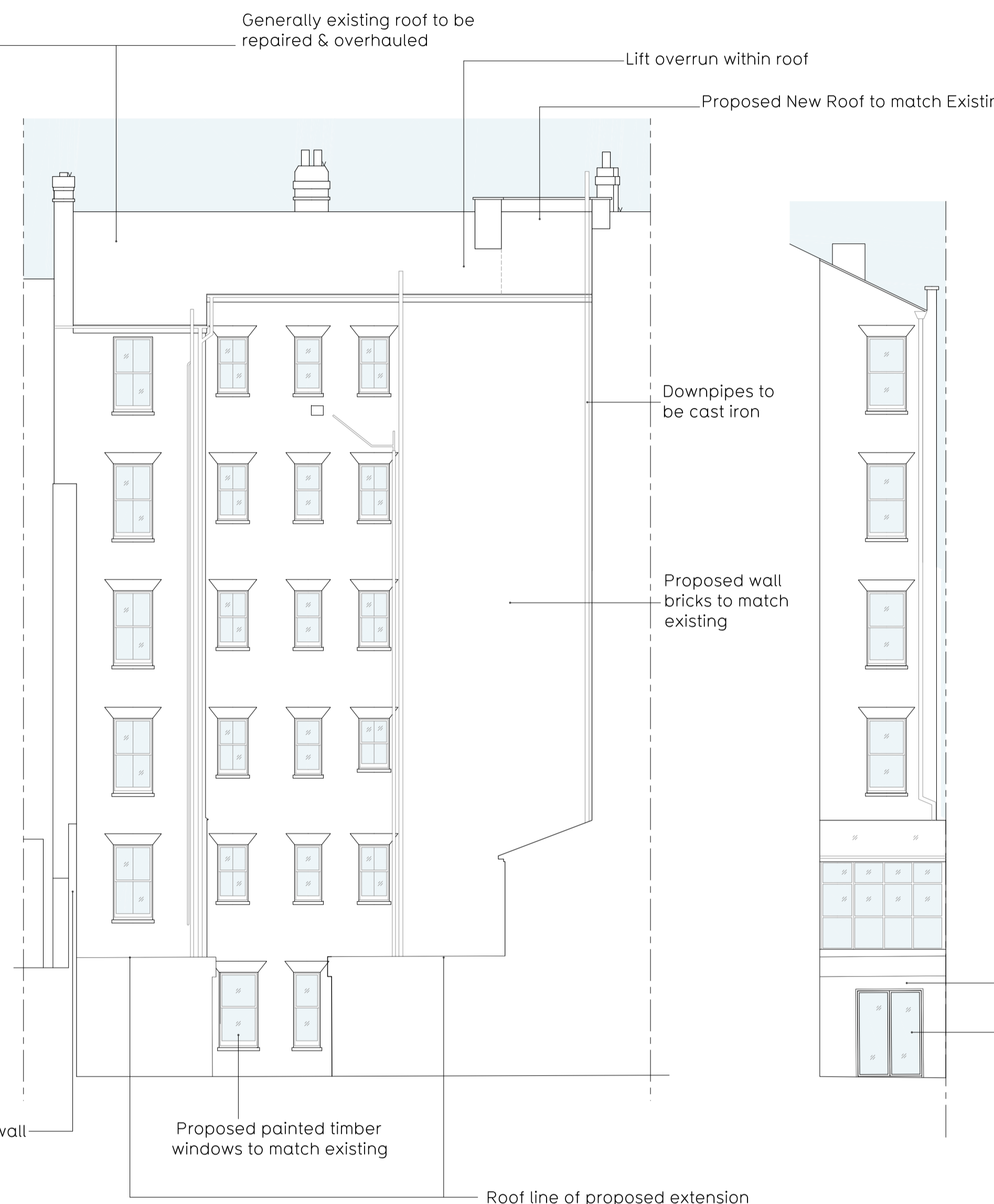
3 Prop. Rear Elevation CC 300 SCALE 1:100
