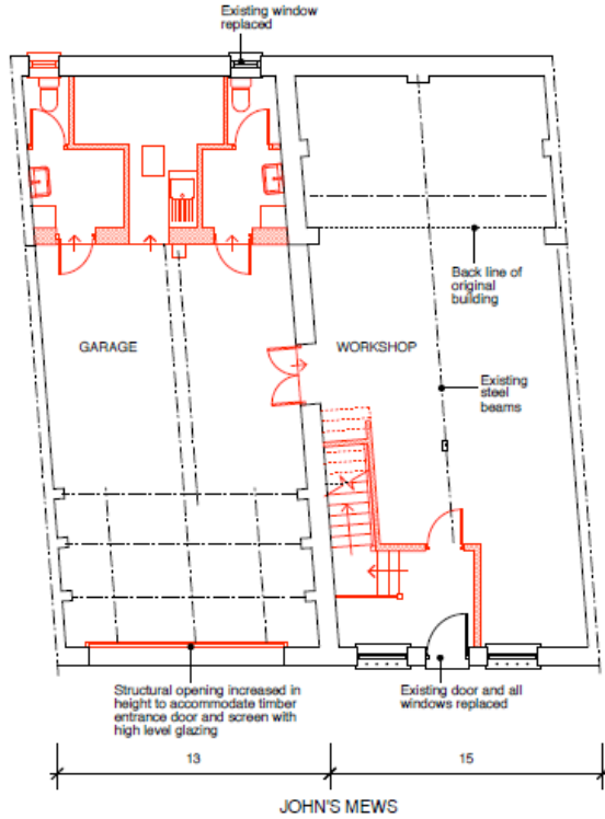
GROUND FLOOR DEMOLITION PLAN
