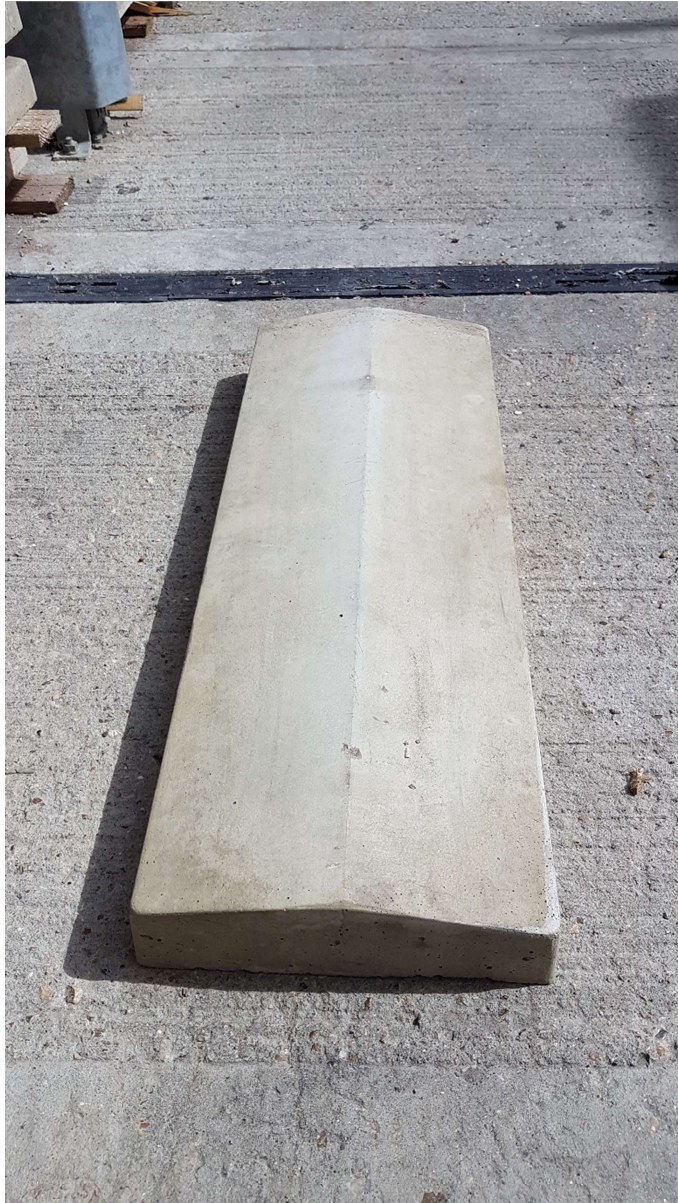
Fig. 3 – Double Weathered Concrete Coping Stone for 225mm Brick To Cap Mansard Flank Walls
