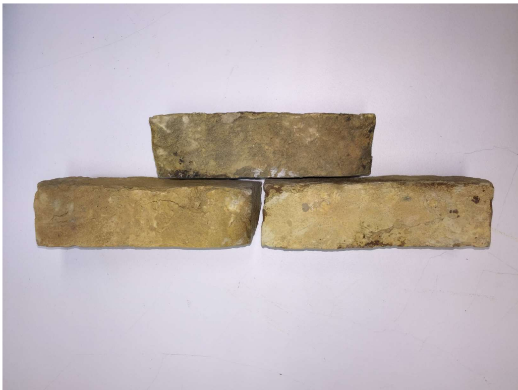
Fig. 2 - London Stock Bricks For Flank Walls of Mansard Roof – colour and pointing profile to match existing
