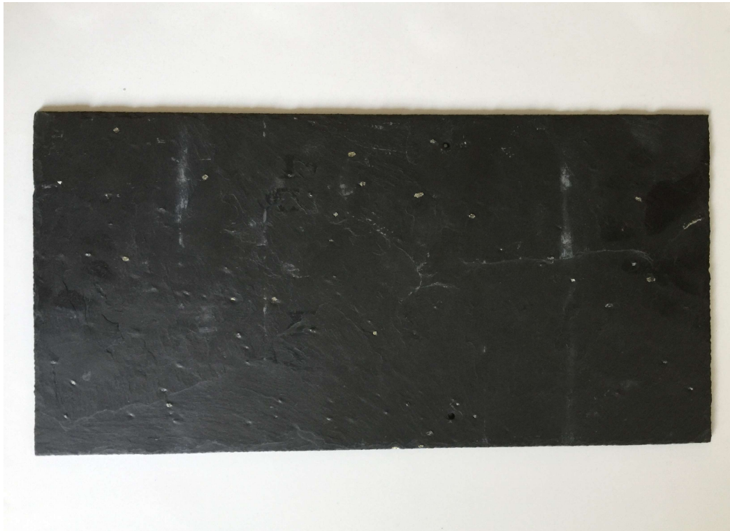
Fig. 1 – Natural Slate - 1 st Quality Spanish Slate, 500 x 250mm
