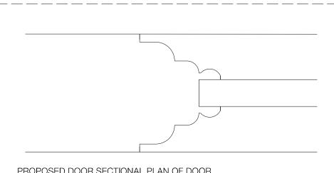
PROPOSED DOOR SECTIONAL PLAN OF DOOR MOULDING PROFILE - Scale 1 : 1
