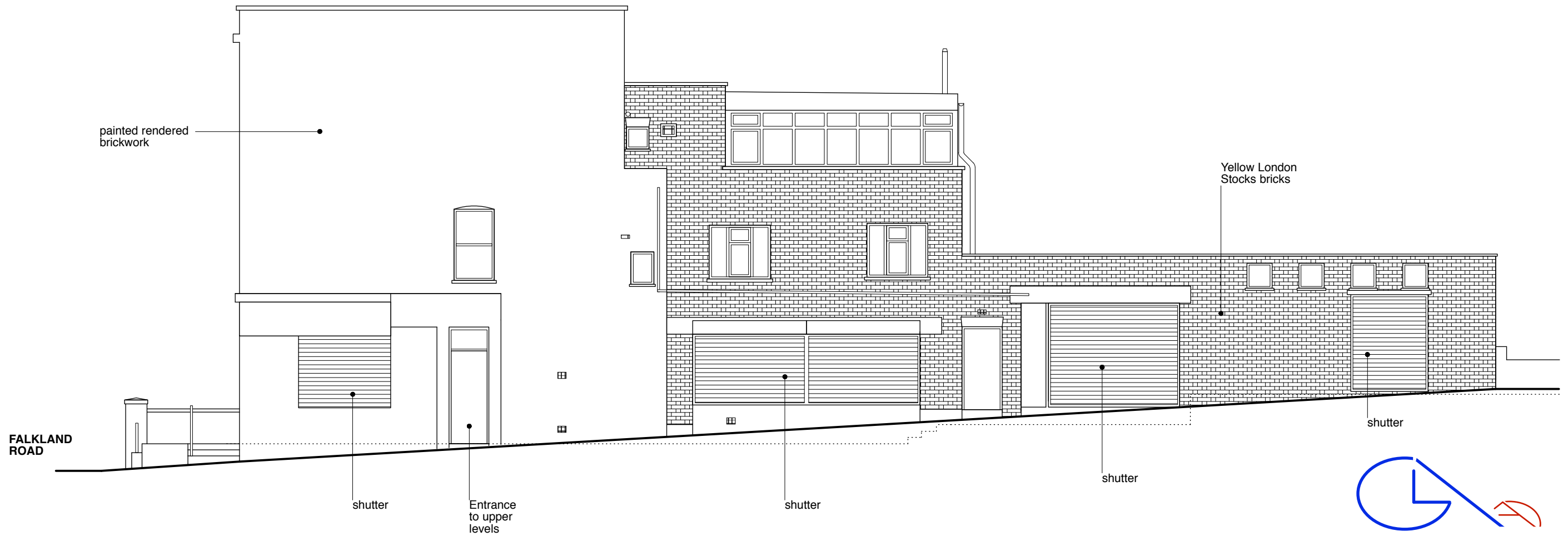
EXISTING SIDE ELEVATION FROM MONTPELIER GROVE scale 1:100
