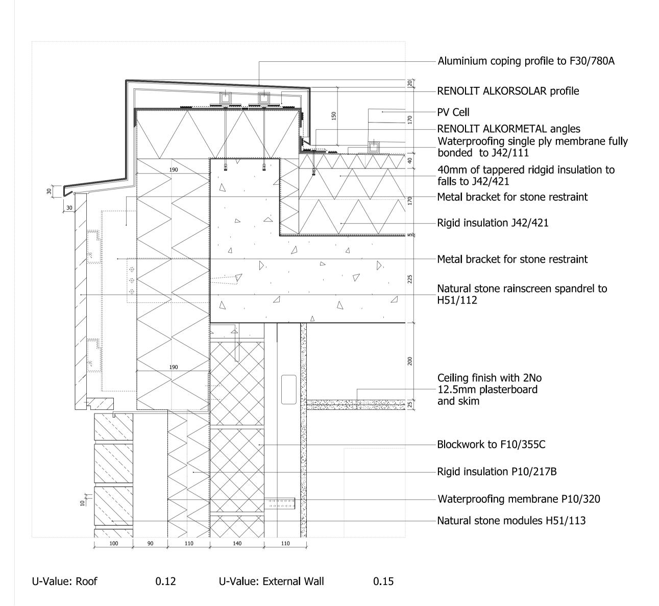
ROOF PARAPET DETAIL OVER RAINSCREEN CLADDING
