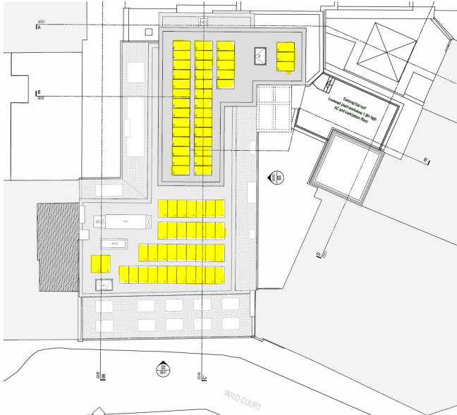
Image shows the propose locations for the PV panels at 8 th and 9 th floors
