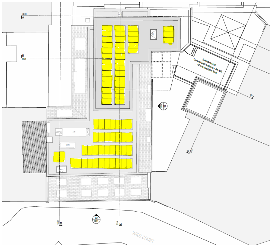
Image above indicates the proposed location for the new PV panels at 8 th and 9 th floors
