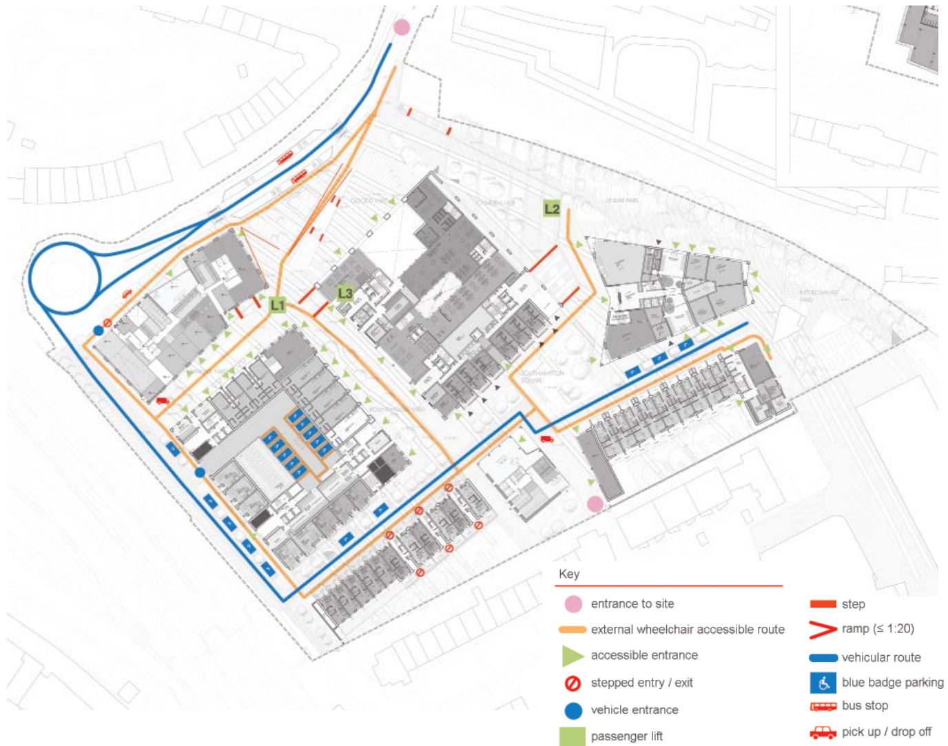
Camden Goods Yard Masterplan indicating means of access, including public lifts (L1, L2, L3), principal gateways and primary access routes.
