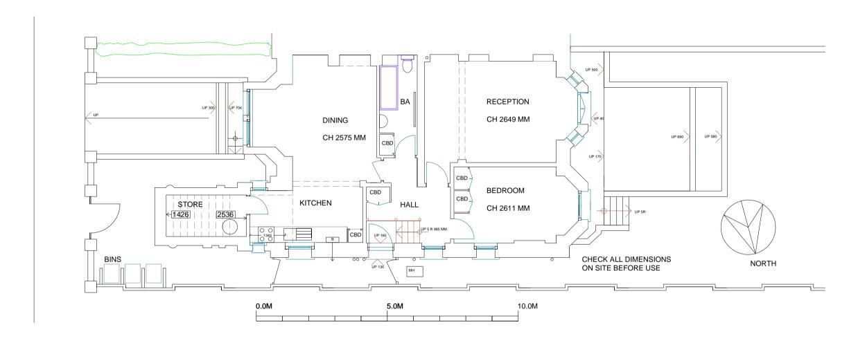
LOWER GROUND FLOOR PLAN AS EXISTING 1:100 @ A3 / 1:50 @ A1
