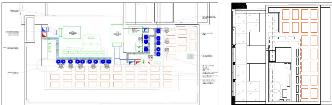
Figure 12: The potential PV layout on both the residential (right) building and commercial (left) building
