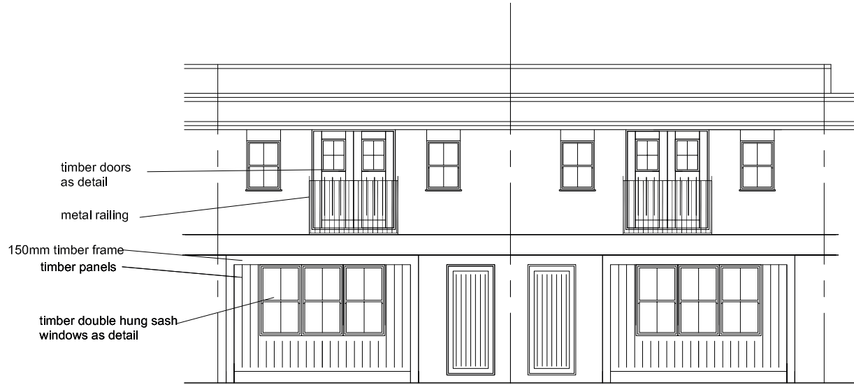
Fig. 12 - Proposed elevational amendments for adjacent building numbers 16 & 17 (application ref: 2016/2446/P) indicating timber panelling to either side of smaller windows.
