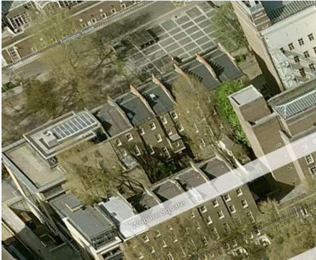
Figure 4.10: Showing the eclectic closet wings to the rear of Nos. 27-32 Torrington Square (Bing Maps). No. 27 appears to include a 3.5 storey closet wing and No. 29's closet wing appears to extend to rear only at 1 st floor level.
