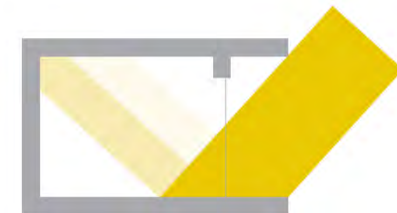
Figure 5. Passive energy measures (deep reveals)
