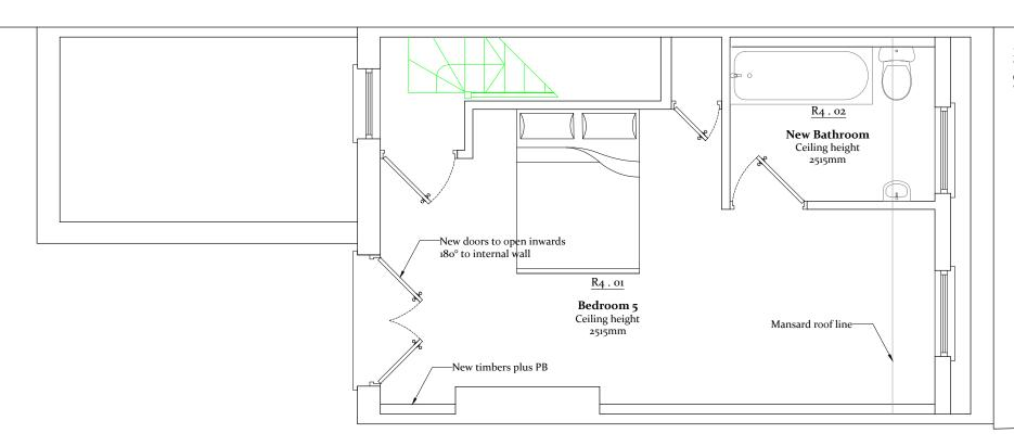
NOTE: DRAINAGE FROM NEW BATHROOM TO RUN THROUGH EXISTING SVP LOCATED ON THE REAR ELEVATION. THIS FEEDS INTO THE MAIN DRAINAGE SYSTEM
