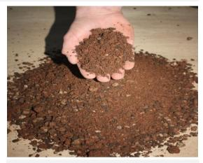
System Considerations: A free draining substrate suitable for use on Intensive and Extensive Roof Systems (Wildflower and Biodiverse) Absorbs and stores water Free draining when saturated Allows root penetration Recycled brick/mineral
