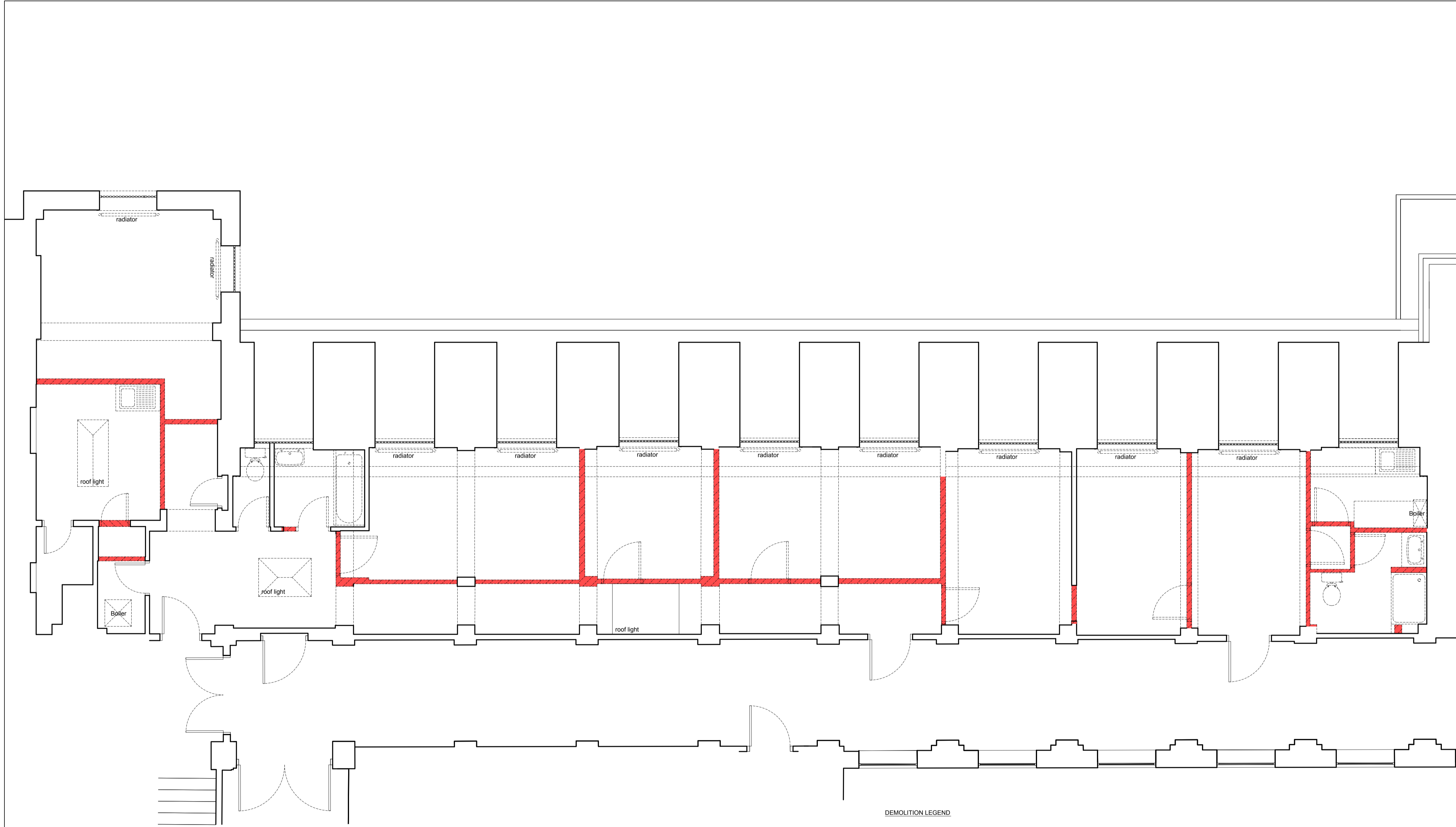
GENERAL BUILDERS DEMOLITION DRAWING
